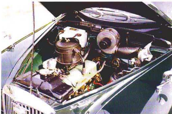
The SC/2 engine, using the export oil-bath filter from the 'YB', but standard fitting to the 4/44
