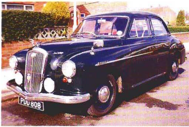
1952 Wolseley 4/44 with MG 'YB' SC/2 engine using a different sump casting, Nuffield hypoid rear axle, and modified Morris Ten/4 series 'M' gearbox, but this time with column gear change. Body is chassis-less, looking like a tall MG 'ZA'.
