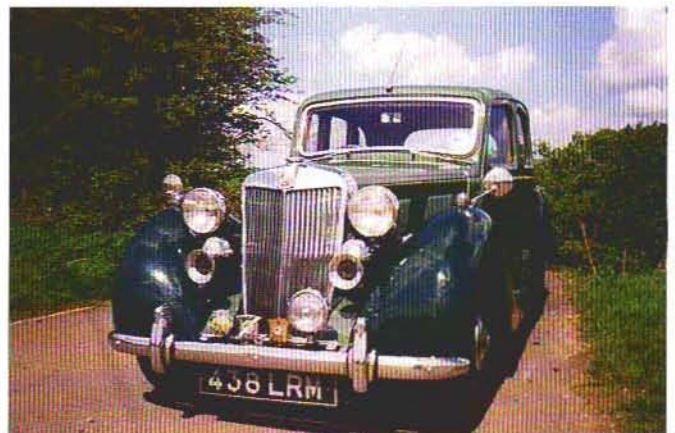
1952 MG YB with the SC/2 XPAG single carburettor engine, Nuffield hypoid rear axle, and modified Morris Ten/4 series 'M' gearbox.
