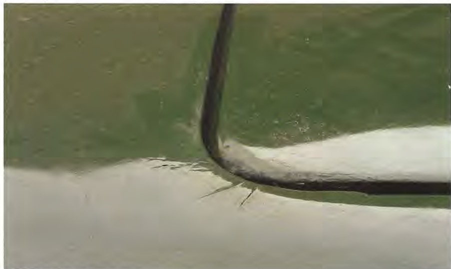
The sunroof cracks.
