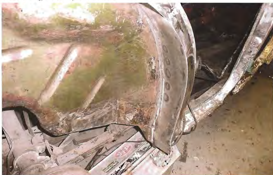
Properly repaired C Post.
