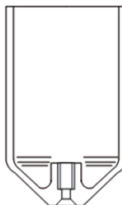
3 - Open up hole for 4 BA screw
