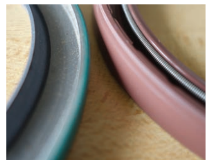
To the left, the kit’s seal that lacks a spring-loaded lip. To the right, the FPM seal with its spring-loaded lip.
