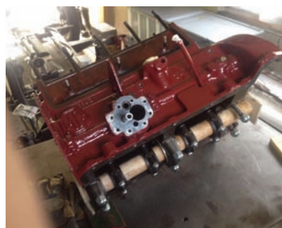
Crankshaft and flywheel removed and con rods secured by piece of round wood
