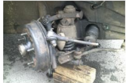
Bent and broken suspension and steering components
