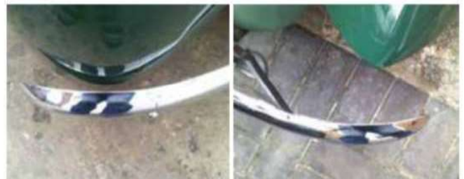
Bumper gaps to wings are educating. Adjustable by adding or removing washers on the body mounting iron
