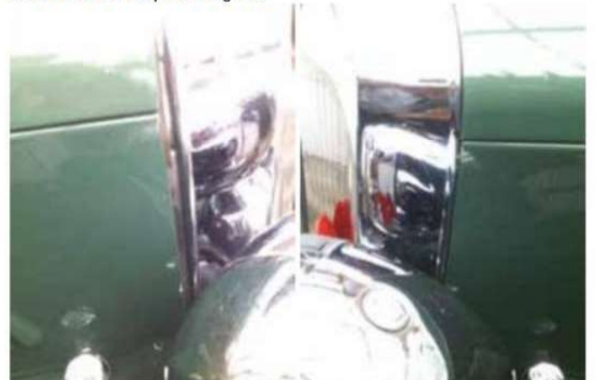
Bonnet to radiator adjustment is by using the bracing rods under the bonnet.
