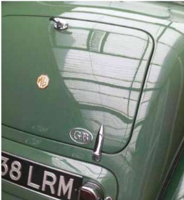
Panel shut lines are important, they can cause wind noise and water leaks if incorrect. The boot and spare wheel panels usually fit properly.
