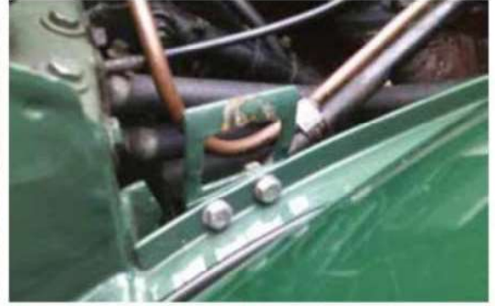
The bonnet locking plates are all handed. Are yours in the correct place?
