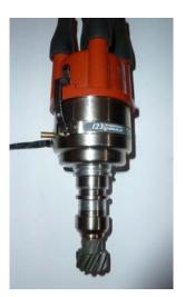
An alternative is to use an external box that connects to the existing distributor, such as the Aldon "Amethyst" Mappable Ignition System,
