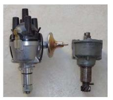
These will fit directly into later TDs and TFs (i.e. those fitted with the D2A4 distributor). However, they will require additional machining modifications in order to fit the earlier XPAG engines using a DKY4A unit. With this distributor distance between the base of the distributor and the drive gear must be increased by approximately 5mm, to accommodate the thickness of the Vernier, and a groove must be machined into the shaft to take the locating bolt.
