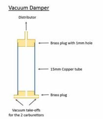
less prone to being affected by pressure pulses.
