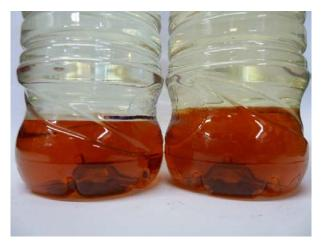
The two bottles in the picture were filled to the same level with red / brown dyed water, the petrol on the left does not contain ethanol and the one on the right does. The difference in height of the water is easy to see. (Note there is nothing at the bottom of the bottle, this is just an effect of the light on the indentation).
