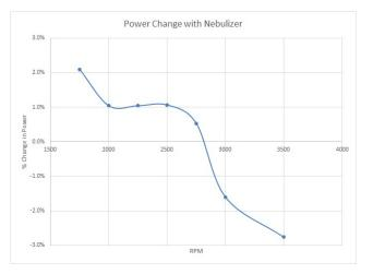
Below 3000rpm, the nebulizer improved power output by around 1% demonstrating benefits of improved fuel atomisation at these engine speeds. Unfortunately, the nebulizer used for these tests also constricted the airflow into the engine explaining power reduction at higher rpm.
