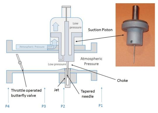
• P1 – where the air flows into the carburettor. This is at atmospheric pressure
