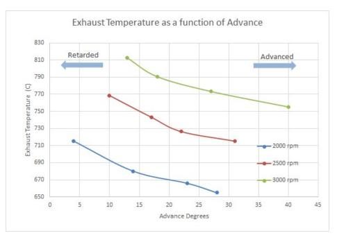
Although there is no data covering throttle settings between half open and fully open, it can be assumed that as the throttle is opened the magnitude of this slow combustion problem will increase until it reaches the level shown by the full throttle tests.
