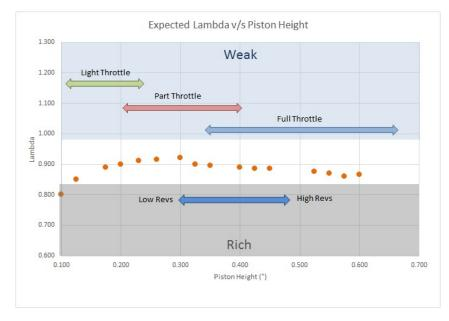
Even though Lambda was set to 0.95 for each test at Manchester, it is possible to calculate what Lambda would have been delivered if the engine had **not** been retuned. The graph below shows this data with the jet adjusting nuts set at 4 flats down from fully closed, running with a standard ES needle and using the same brand of 95 octane petrol.
