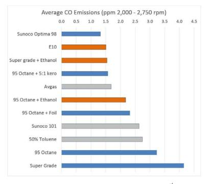
the diagram shows the average CO levels in the exhaust gas for each fuel or combination for these tests. The lower the levels of CO, the better that sample of fuel is burning. The grey bars show the special fuels we tested and the orange bars the ones containing ethanol.
