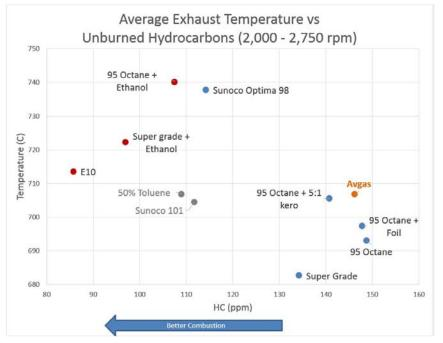
and 95 Octane + 5:1 kero both burn better than the 95 Octane on its own. Adding kerosene certainly improves the combustion suggesting any fears it will not burn are unfounded.
