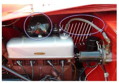
engine, not the best place. For example, although not original, pancake filters fitted directly to the carburettor inlet that draw colder air from the slits in the bonnet would be better.
