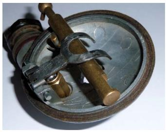
a fuel level of 3/16" below the jet bridge (approximately half way between 1/8" and 5/16" recommended in the factory handbook for the TC). The original brass floats weigh 24gm which gives a petrol level below the jet bridge of 3/8" (as normally specified for SU carburettors).
