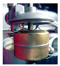
Should you adjust the forks, it worth inserting a pencil through the hole in the lid and the centre of the float to check it does not foul the pivot support (highlighted on the picture by the red circle) before the needle valve shuts off.
