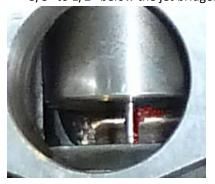
heavier floats to give a fuel height of 3/16" below the jet bridge. The latter tests showed an average increase in power output around 5% for three different fuels, however, this figure should be taken with caution as these tests were run many months apart and other factors may have influenced the measurements.
