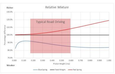
Over the normal range of piston heights used for driving on the road, the *ES* needle can be used in all three cases. Carburettors fitted with a blue spring can be made richer by screwing out the jet adjusting
