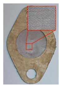
The reason a foil like this is not practical for normal driving is that unless the air and petrol entering the engine can be filtered to remove any particles greater than 8 micrometres in diameter, such a foil would soon block and choke the engine.
