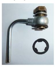
breather pipes allowing the air pressure in the float chamber to remain at atmospheric.
