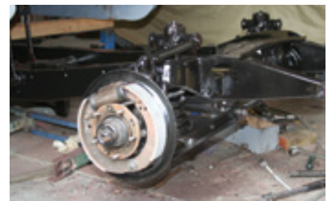
Front brakes with double-acting shoes.
