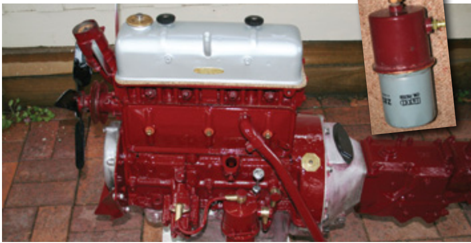
The completed engine and gearbox. Inset: the oil filter before painting.
