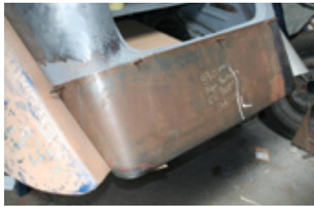
New rear panel pinned in place.
