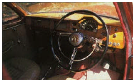
ZA fascia looks like fifties radio set with half octagonal speedo. Early Bseries 1½ litre engine gives willing 60 bhp, with twin SUs supplying the mixture.
