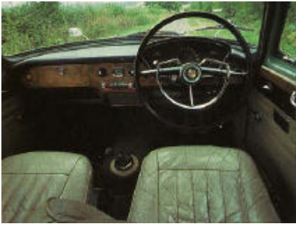
Farina Magnette interior is best part of car with characterful instrument cluster, walnut on dash and doors and hide-covered seats.
