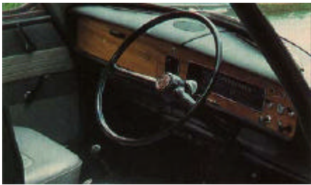
1100 interior has strip speedo but no rev counter. A willing A-series in 1100 gives mild performance but is willing unit.
