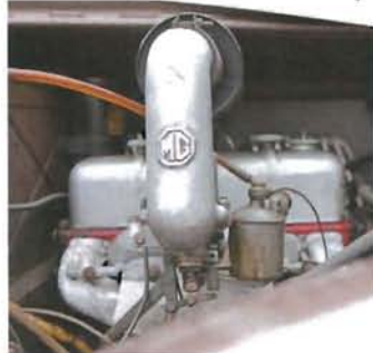
Engine in the Y-Type was a 46bhp 1250cc XPAG, which had a lot of weight to lug about – including an in-built Jackall system.
