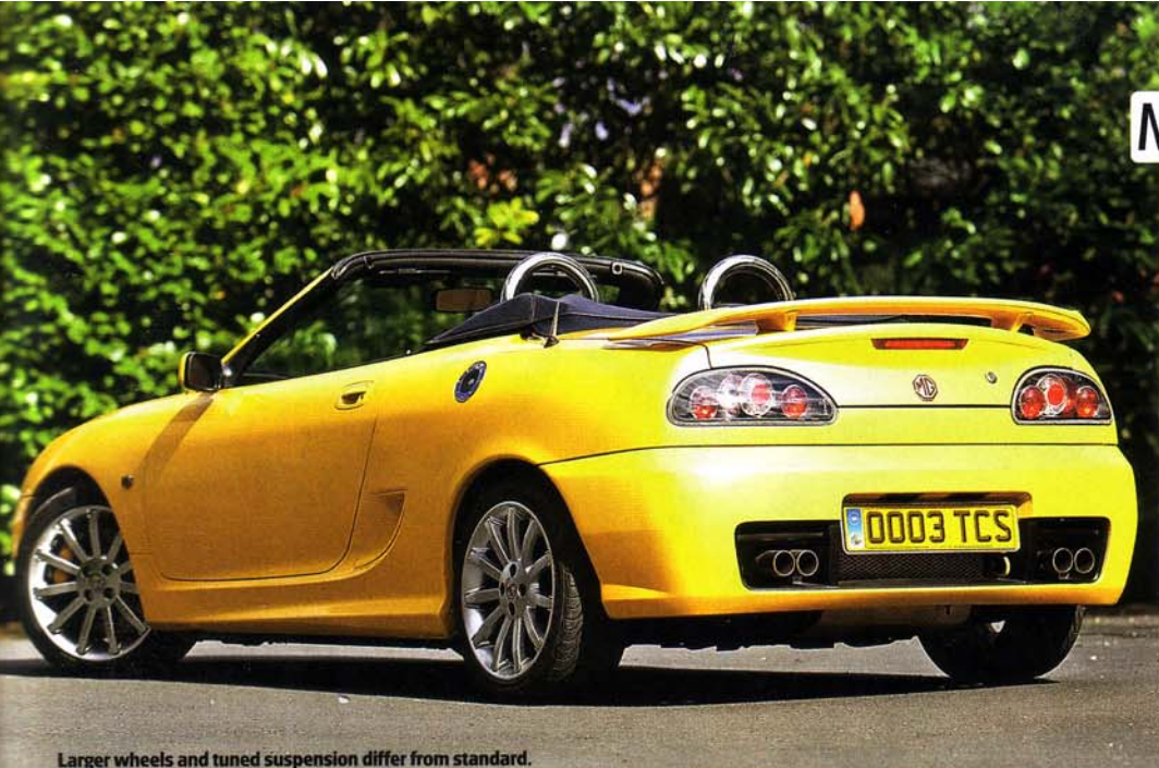
Larger wheels and tuned suspension differ from standard.
