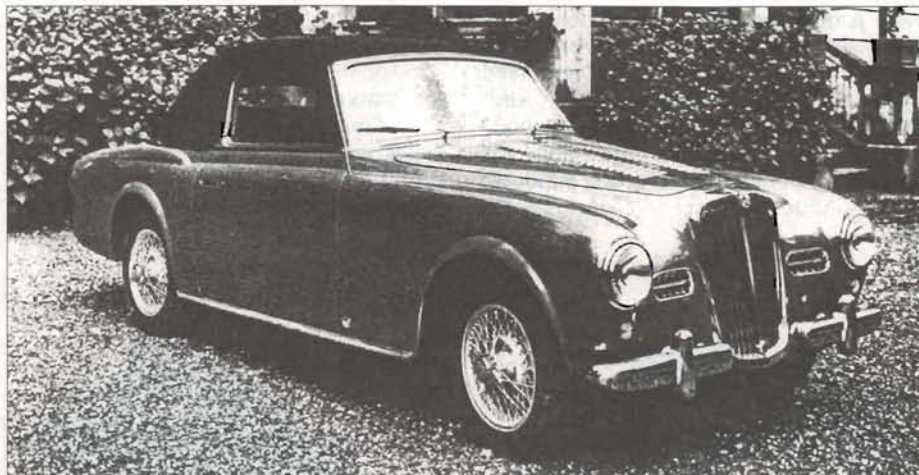
The Castagna 2/3 seater drop-head coupé body fitted to a TD chassis for Roger Barlow. The performance was disappointing and on his return to Los Angeles he had Al Moss fit a supercharger
