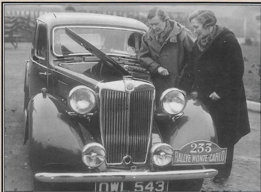
Betty Haig and Barbara Marshall with their Y-type before the 1950 Monte Carlo Rally. Note the 'clearview' panel in front of the driver and the electric defroster in front of the passenger. Saloon cars of the period had poor heating and demisting systems and Winter travel meant frozen windscreens and poor visibility.
