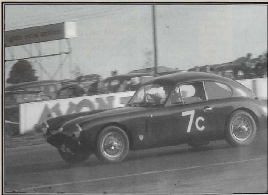
The last YB chassis from the factory was used by Dick Jacobs for this special seen here racing at Silverstone in the 6 hr. relay race in 1954. The engine was tuned to TD MkII specification and the body was constructed of fibreglass over a steel tube framework.
