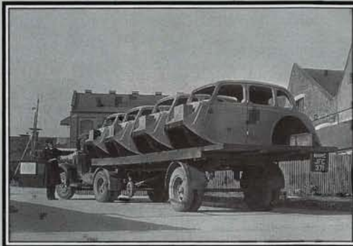
Outside, in the factory yard, completed bodies arrive and await their turn to be hoisted to the 'top deck' where they were readied for fitting to their chassis. Right up to the close of the factory this was the route taken by the Midget and MGB bodies, although only the Midget required trimming as MGBs arrived fully trimmed and with weather equipment fitted.
