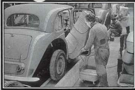
Working towards the end now and with the bumpers fitted the seats are installed. The various trim and colour combinations meant that each car had to carry a job sheet listing the final specification.
