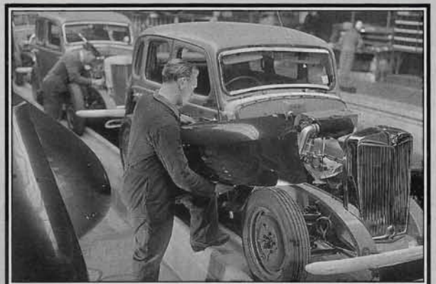
Almost ready for final inspection and the bonnet and headlights are fitted, the wiring connected up, petrol added to the tank and the car is then driven away for road test. Note the inspector or foreman in his white coat.
