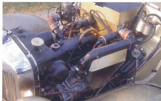
The powerhouse: intercooler sits in big square housing on bulkhead
