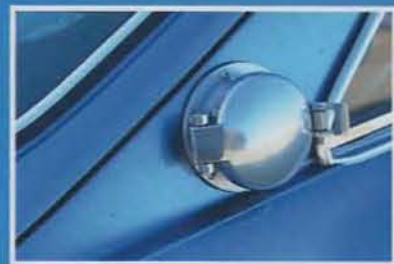
ABOVE: The obligatory quick release fuel filler has been located on the righthand side C-pillar.
