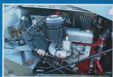
ABOVE: The XPAG engine has been enlarged slightly to 1347cc and given a number of other tweaks during a rebuild completed in 2005.
