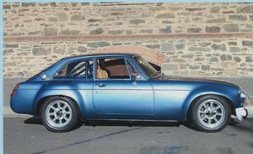
ABOVE/BELOW: The same attention to detail has been applied to the interior as to the exterior – those flared Sebring arches were fabricated in steel and welded on.
