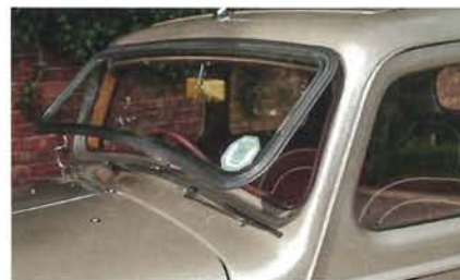
ABOVE AND LEFT: An opening screen and an in-built Jackall system were both carry overs from the 1930s.
