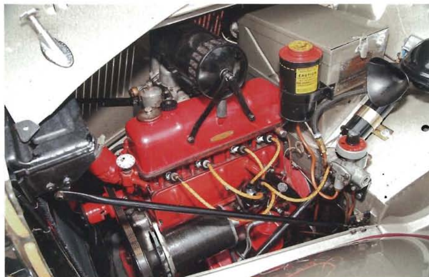
ABOVE AND LEFT: Power for the YB came courtesy of a 1250cc OHV XPAG engine making 46bhp at 4800rpm.
