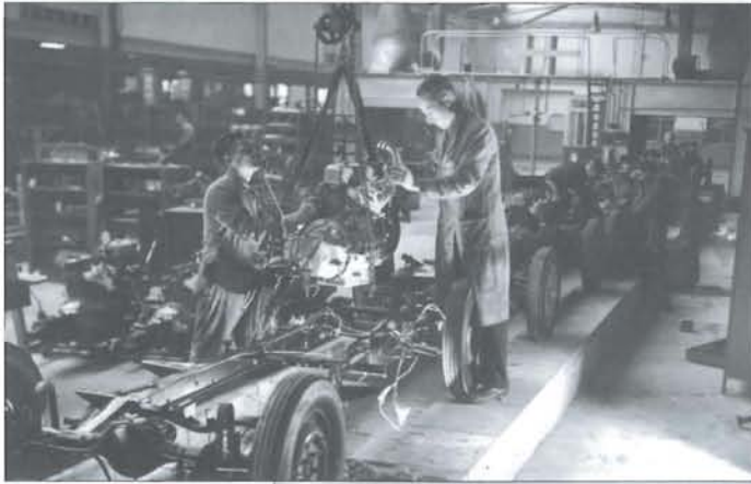
Above: The engine and gearbox were fitted as a unit to the rolling chassis.
