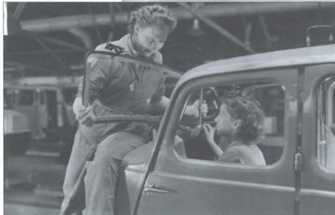
Left: Two people were needed to fix the windscreen frame to the body; this was top hinged so it could be wound open in hot weather. For this reason the windscreen wiper arms were fitted with knobs to stow them on the scuttle, below the windscreen frame. Right: Once the windscreen wiper mechanism was fixed in place the wooden dashboard with its attractive veneered finish could be installed.
