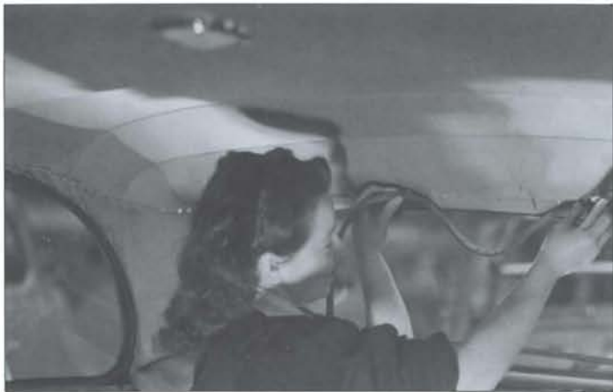
Above: One of the trimmers installs the seal around the rear window. Above right: The door lining panel is installed. The interior of the Y-type was well finished and was one of the most appealing features of the model. Right: As anyone who has ever attempted the task will testify, installing a headlining is not the easiest of tasks. Below right: One of the final jobs to be completed on the top floor is the installation of the seat squabs.
