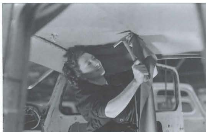
Above: One of the trimmers installs the seal around the rear window. Above right: The door lining panel is installed. The interior of the Y-type was well finished and was one of the most appealing features of the model. Right: As anyone who has ever attempted the task will testify, installing a headlining is not the easiest of tasks. Below right: One of the final jobs to be completed on the top floor is the installation of the seat squabs.
