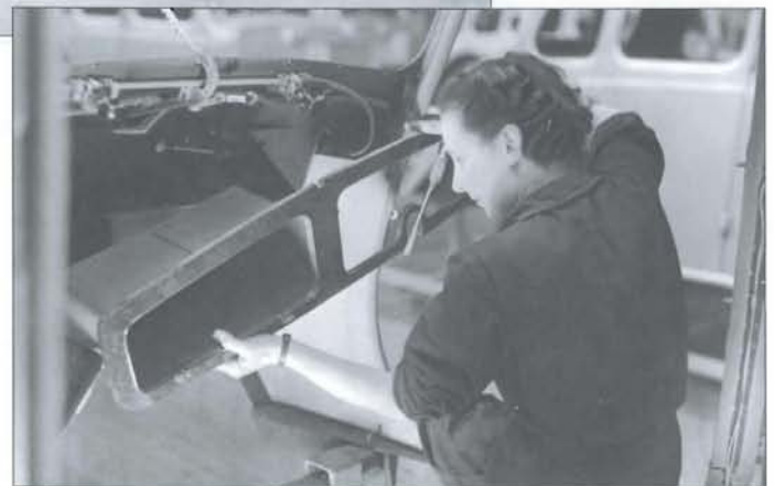
Left: Two people were needed to fix the windscreen frame to the body; this was top hinged so it could be wound open in hot weather. For this reason the windscreen wiper arms were fitted with knobs to stow them on the scuttle, below the windscreen frame. Right: Once the windscreen wiper mechanism was fixed in place the wooden dashboard with its attractive veneered finish could be installed.
