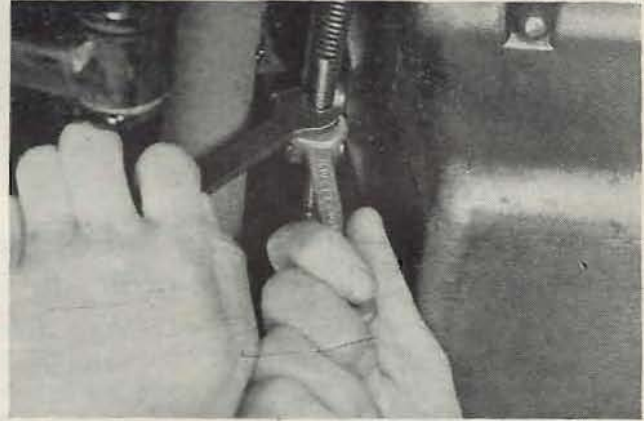
2. To obtain this, release the locknut at the forward end of the clutch operating cable.
