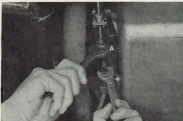
5. To obtain this adjustment, grip the stop nut and slacken off the locknut A.
