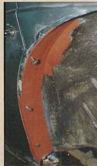
The worst part of the wheel-arch has now been repaired.
