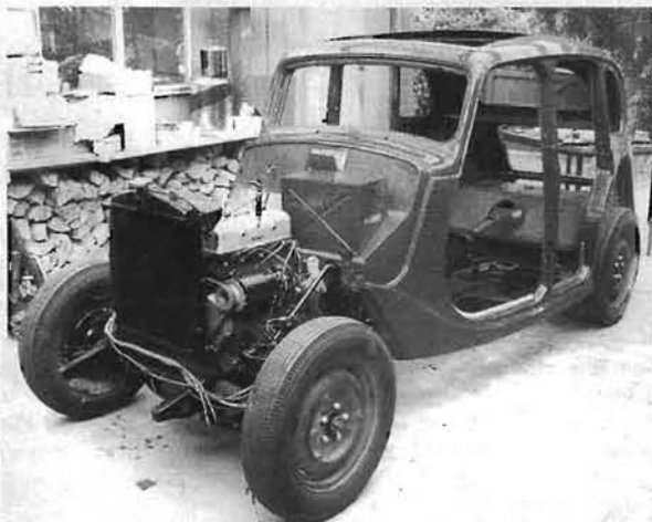
TOP LEFT. The independent front end with rack and pinion steering and forward mounted sway bar.
